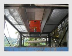
Automatic bunker cover with lower opening, positioned under the plates pack, to collect the drops caused by the filtration and the eventual clothes washing
